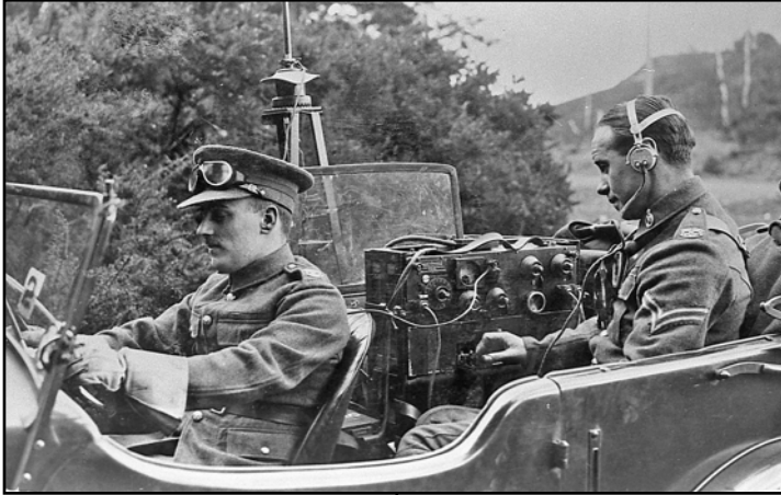
Range trials of the Dial System were conducted in 1932. One of the stations was carried in a Morris Eight light car. This photo shows a standard No. 1 Set installation in this vehicle without the Dial System attachment.
